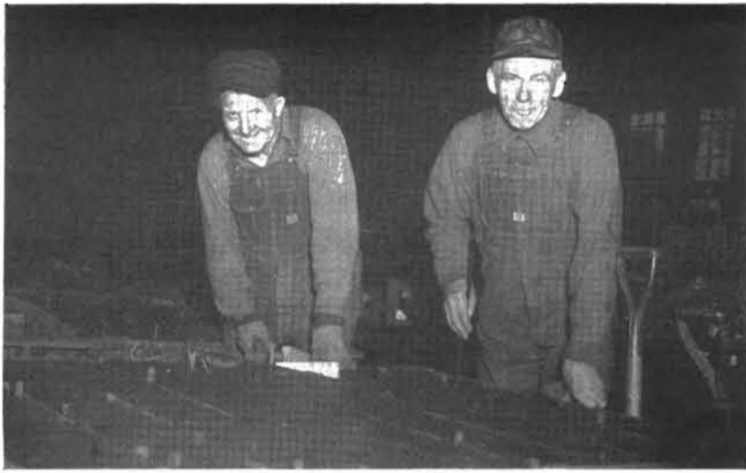
Horace Barrett and Charles Larson, molders, clamping a mold.
