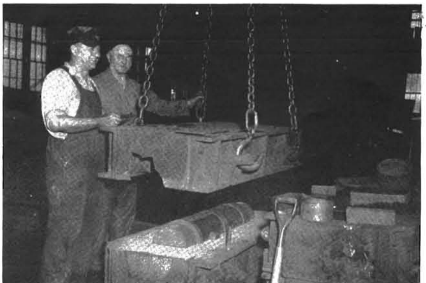
William Vogeler and Clarence Dunn, molders, closing up a mold.
